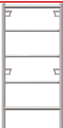
B-FL27W5HX27L6 27.5"Wx5'H Ladder Frame X-Lk 27-3/4" Lk Spacing 21.2 lbs.
