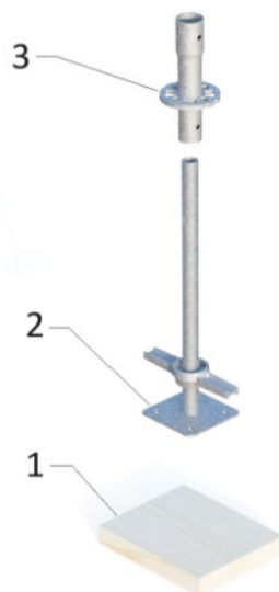
Figure 14 - Scaffold Tower starter
