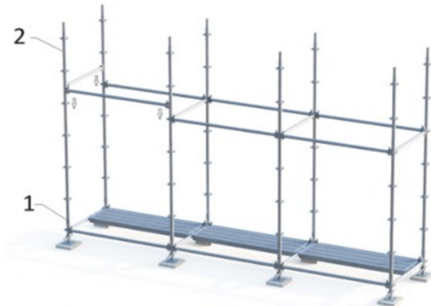
Figure 17 – Standards and Ledgers Installation for Scaffold Levels
