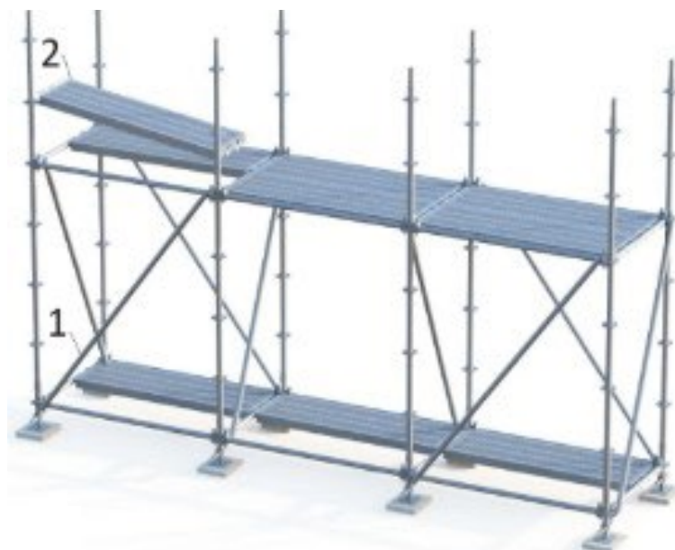
Figure 18 – Planks and Diagonals Installation for Scaffold levels
